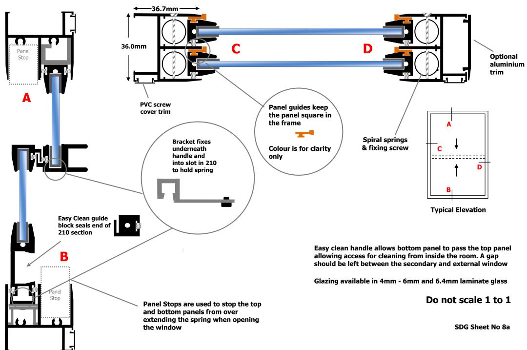
Secondary Glazing Easy Clean Spring Counterbalanced Vertical Slider
